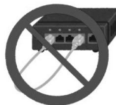
**Do not use old hubs or broken LAN cables**
